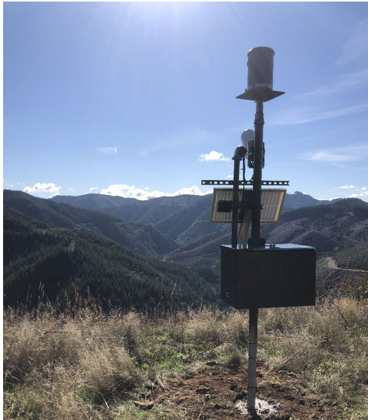
Figure 3.3. New precipitation gage at Willapa Hills.
