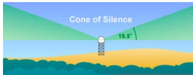
Figure C.5. Radar cone of silence.
