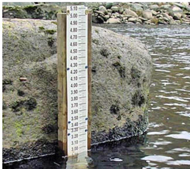
Figure C.8. Staff gage. Image from USGS.
