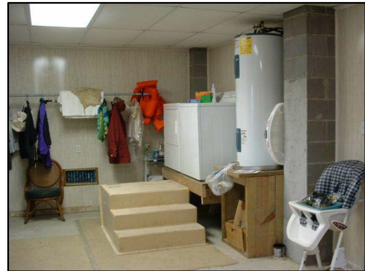
Wet floodproofing floodable areas
