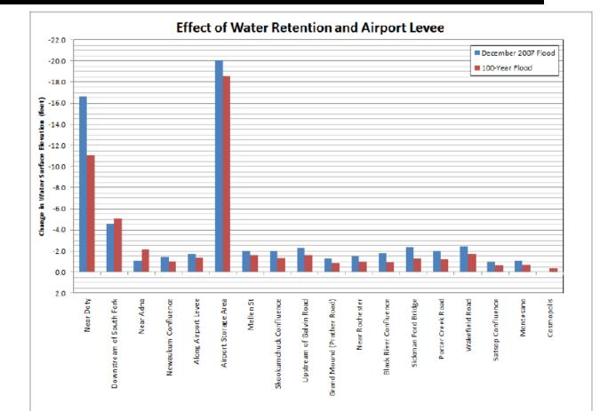
Figure 2: Predicted Changes in Water Surface Elevations from Water Retention and Airport Levee
