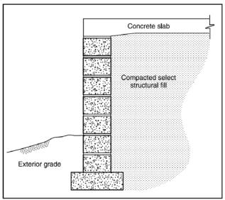
Figure 8. Back-filled stem wall foundation (openings not required)
