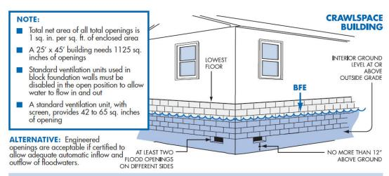
Solid perimeter wall foundations can enclose flood-prone space. A crawlspace is a good way to elevate just a couple of feet. In all cases, the following are required: openings/vents, elevated utilities, flood resistant materials, and limitations on use.
