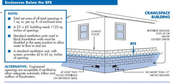
Solid perimeter wall foundations can enclose flood-prone space. A crawlspace is a good way to elevate just a couple of feet. In all cases, the following are required: openings/vents, elevated utilities, flood resistant materials, and limitations on use.
