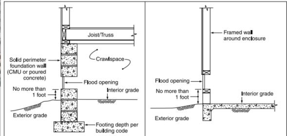
Figure 1. Typical enclosures with flood openings
