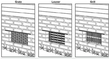
Figure 15. Typical Flood Opening Covers (source: FEMA)
