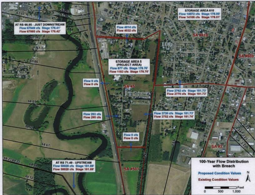
Figure 6. Hydraulic results for the 100-year event assuming traffic barriers breached.
