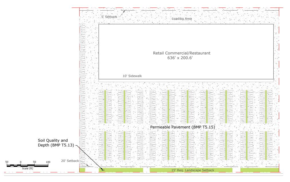
Figure 44. Scenario 13. Permanent Stormwater Site Plan – Large Commercial Development, 2012 Requirements, Outwash Soils
