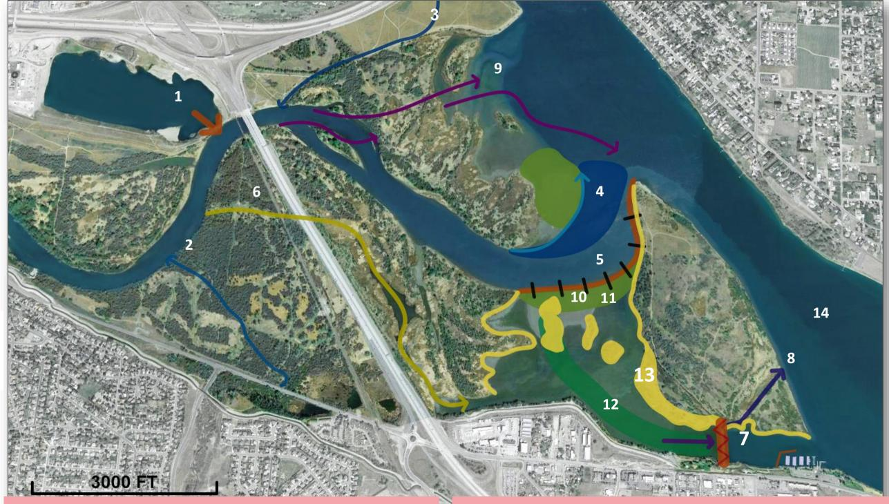
Measure 7: Complete or Partial Removal of Causeway to improve flow through the backwater. Retained
