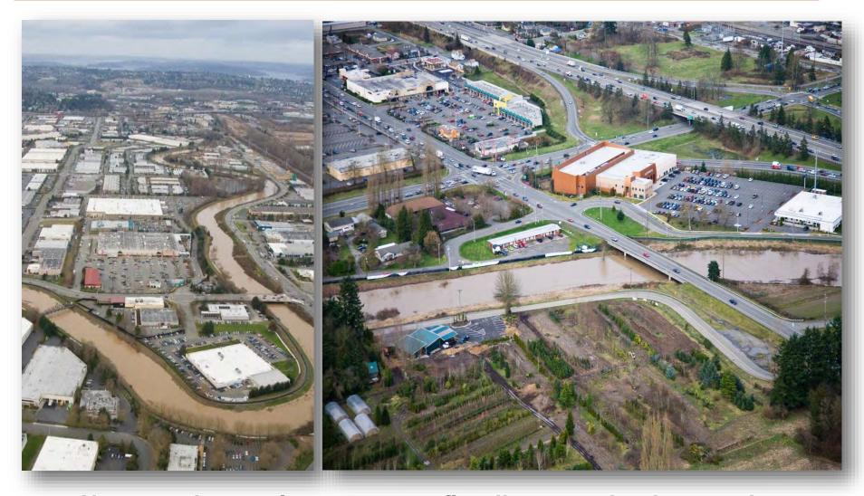
Near-continuous levee system, flooding contained, extensive
