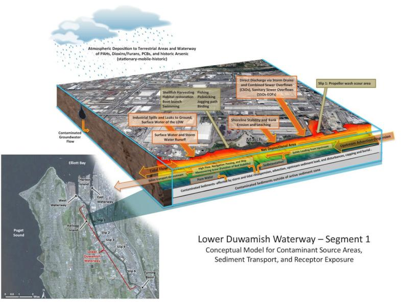
Figure 2-4. Conceptual model for contaminant source areas, sediment transport, and receptor exposure in a portion of Segment 1 (RM 0.3 to RM 1.2)
