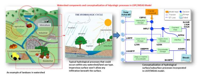
Figure 5-1. Hydrologic component of the LSPC model
