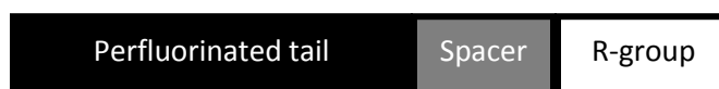
Figure 6 Schematic of a fluorinated surfactant. The perfluorinated chain is represented by the black bar (left), the non-fluorinated hydrocarbon spacer by the gray portion (center), and the functional R-group (right) by the white portion. The R-group is adjusted to ensure solubility in the solvent of interest or other functional purposes.
