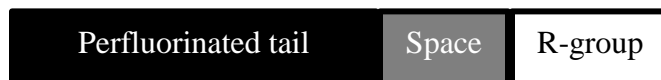
Figure 6 Schematic of a fluorinated surfactant. The perfluorinated chain is represented by the black bar (left), the non-fluorinated hydrocarbon spacer by the gray portion (center), and the functional R-group (right) by the white portion. The R-group is selected to ensure solubility in the solvent of interest or to confer other functional properties.
