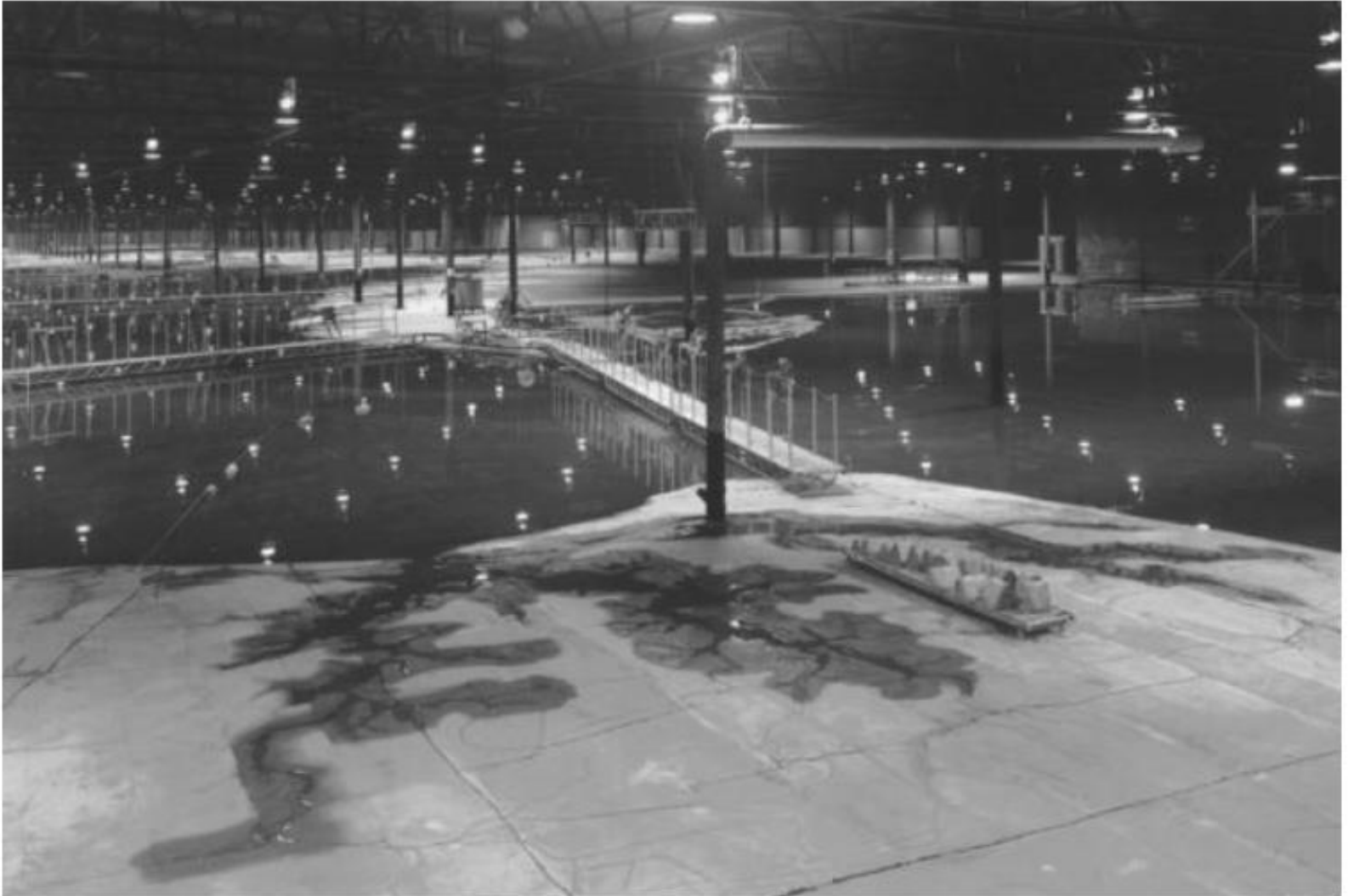
Chesapeake Bay Model, as it looked in August 1977. U.S. Army Corps of Engineers Waterways Experiment Station photo
