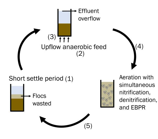
Key selection pressures 1. Short batch settling keeps mainly fast Settling granules (0.5 – 3 mm typical)
