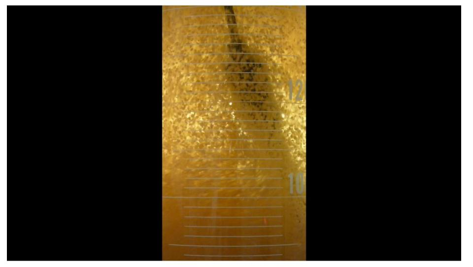
Advantage #2: Anaerobic-aerobic operation provides granules with Enhanced biological phosphorus removal (EBPR) and simultaneous nitrification/denitrification (SND)
