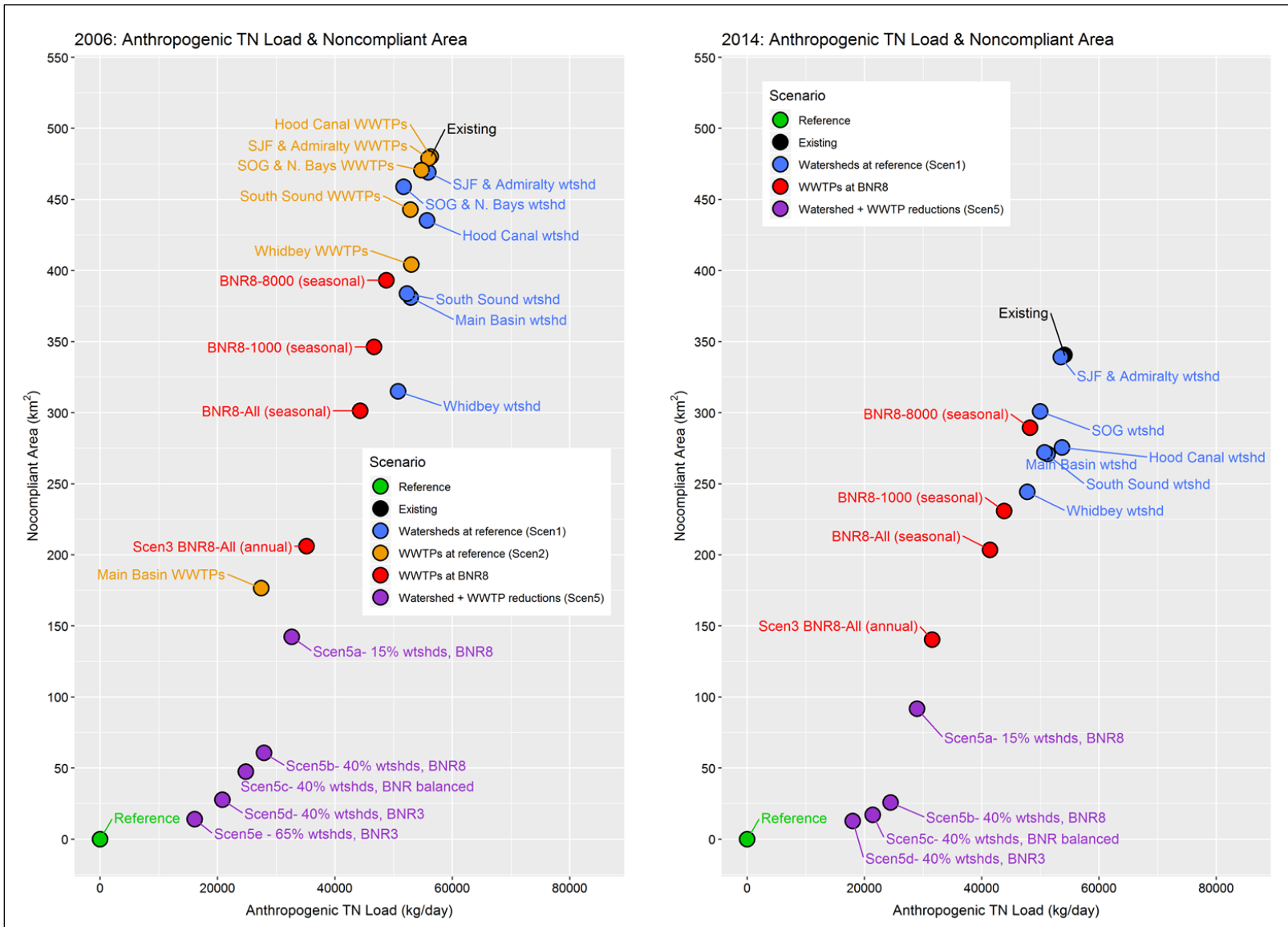
Figure 8. Comparison of predicted noncompliant area in WA waters of the Salish Sea resulting from all Optimization Scenarios and BNR8 Scenarios, with each scenario's associated anthropogenic total nitrogen loading in 2006 (left) and 2014 (right).
