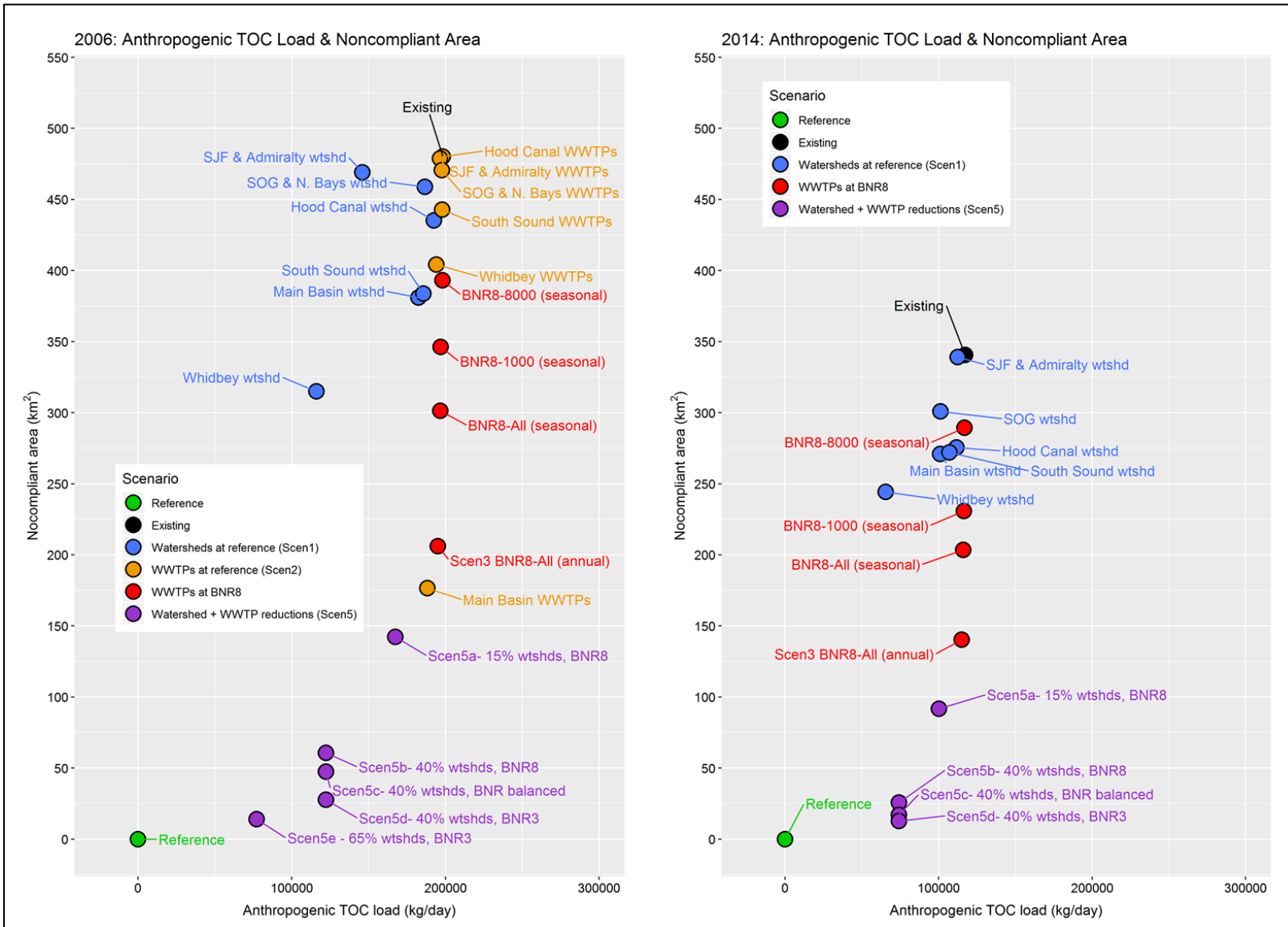
Figure 10. Comparison of predicted noncompliant area in WA waters of the Salish Sea resulting from all Optimization Scenarios and BNR8 Scenarios, with each scenario's associated anthropogenic total organic carbon loading in 2006 (left) and 2014 (right).
