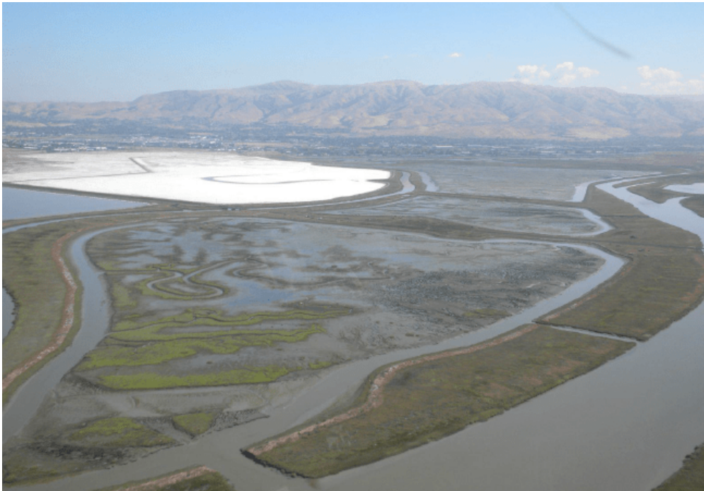
Fig. 5.6: Visualization of the bathymetry database assembled for modeling Lower South Bay. A 2m master bathymetry map, targeting the hydraulic configuration of the sloughs and ponds, has been completed for the study area. A portion of the Island Ponds is shown from a Cris Benton kite photo (left) and in a rendered bare-earth view of the bathymetry database (below).
