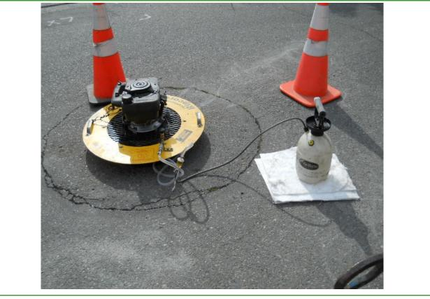
Smoke testing engine and liquid smoke in place during smoke test (Photo Credit: City of Seattle).
