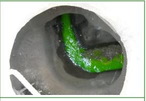
Dye test from a home thought to be illicitly connected to the storm drainage system (Photo Credit: City of Seattle).
