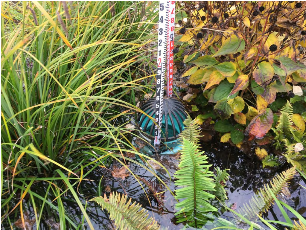
Above photo: Cell M3Q inlet modified for monitoring and nearby well points and ponding station. Lower Photo: close up of overflow structure during infiltration testing.
