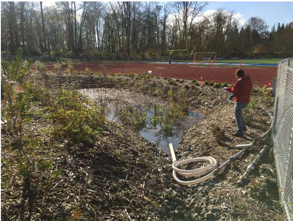
Cell MPP overview during infiltration testing.
