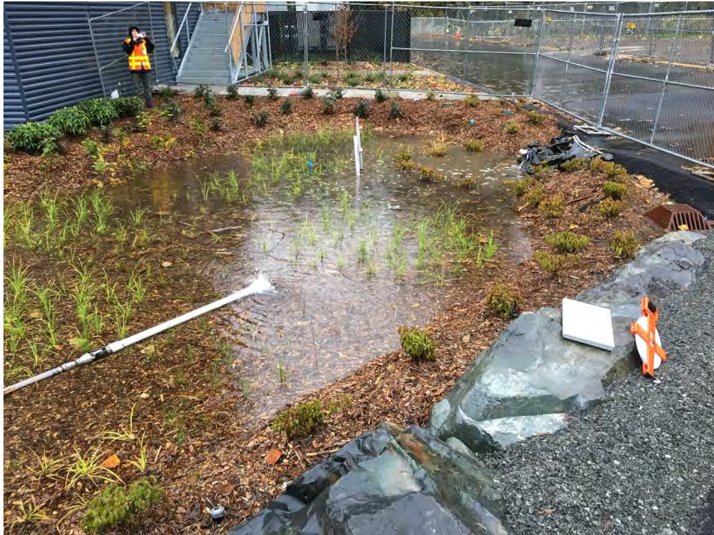
Cell SSW overview during infiltration testing.
