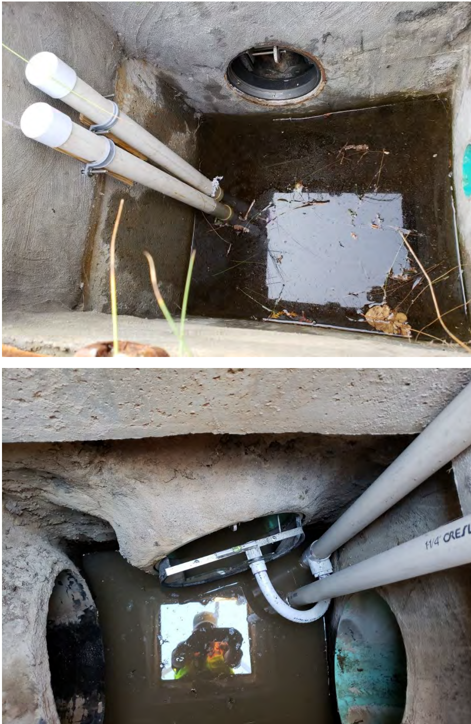
Figure 4. a) Outflow Monitoring in Catch Basin at BUW and b) Outflow Monitoring in Outlet Structure with a Stilling Well at FWI
