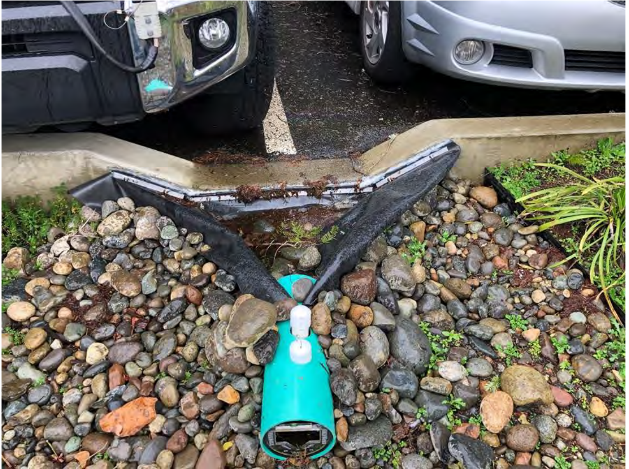
Figure 3. Inflow Monitoring in Curb Cut at FWI_IN2
