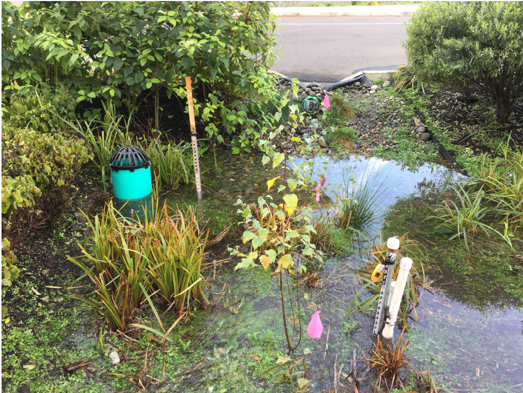
Above photo: FWI during infiltration testing. Overflow beehive not visible in vegetation, located in lower left. Lower Photo: overflow structure and staff gauges.
