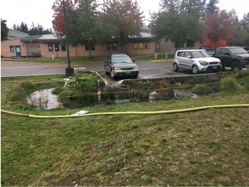
Cell TBM during infiltration testing, looking southwest, after about 6.5 hours of inflow.
