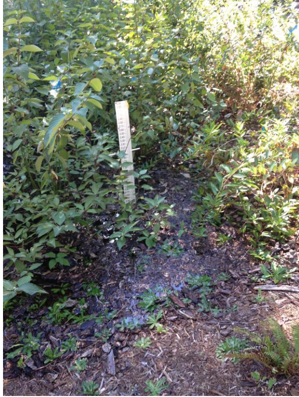
Cell SLP "I" during infiltration testing, with SG-2 visible
