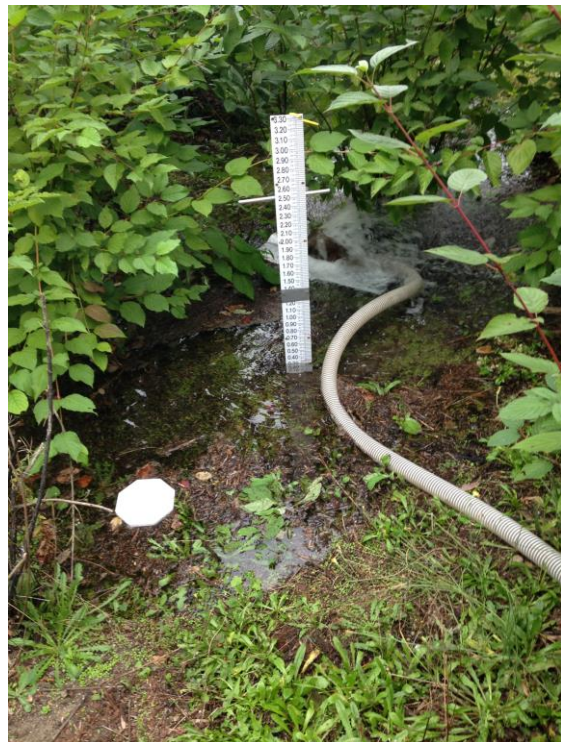
Cell NOL SG-2 during infiltration testing, with nearby underdrain cleanout (white PVC octagonal cap)
