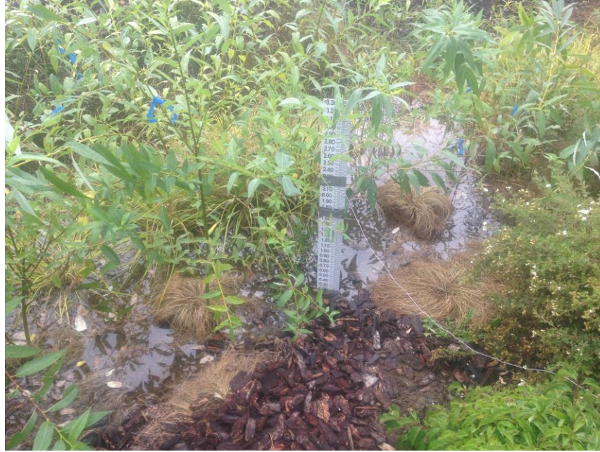
Cell ORLA2-B during infiltration testing, with SG-1 affixed to well point
