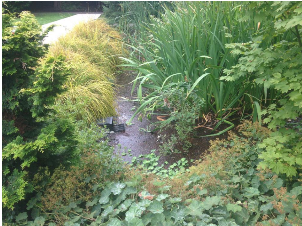
Cell MCCA2 during infiltration testing (overflow grate opened for observation)
