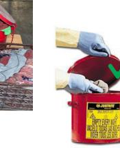
Engine parts: remove residual automotive fluids and store separately (don't mix wastes).
