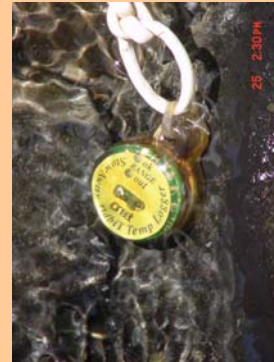
Onset Computer Corporation TidBit Temperature Logger downloaded once per month
