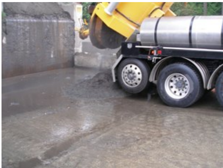
Vactor truck dumping its load at a decant facility for proper waste handling.
