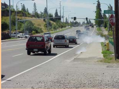
Smoke identifies location of stormwater catch basins on Enchanted Parkway
