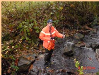
SWM staff calculating total stream discharge in West Hylebos Creek using a hand-held current velocity meter
