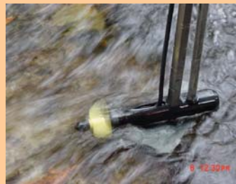
Close-up of current velocity meter
