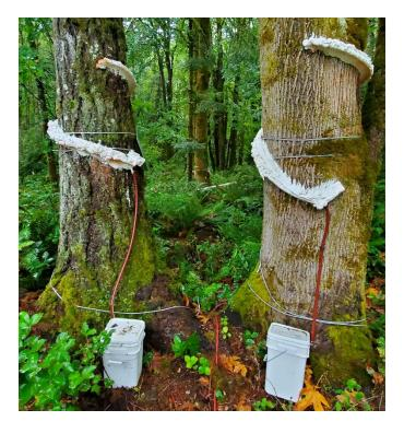
Figure 7: Stem flow buckets placed beneath stem flow collars on a Douglas-fir (left) and bigleaf maple (right).
