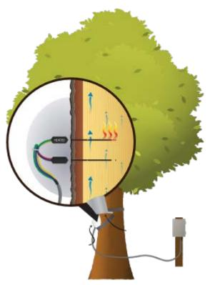
Figure 3: Upper sap flux probe that is heated and measures temperature dissipation, while lower probe measures ambient sap temperature. The temperature difference between the two probes is dependent on the rate of sap transported up the xylem.
