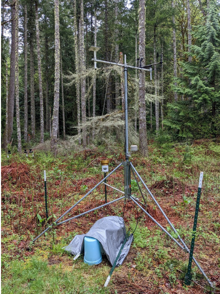
Figure 5: One of two weather stations located near sites 1 and 2, equipped with an open-canopy rain gauge, relative humidity sensor, temperature sensor, wind speed and direction sensor, leaf wetness sensor, and barometric pressure sensor.
