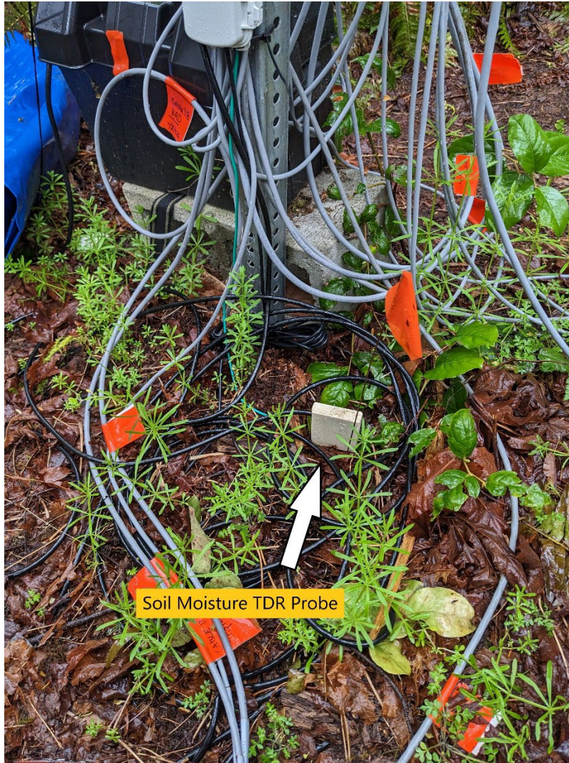
Figure 2: Soil moisture at sites 1 and 2 is continuously monitored using time domain reflectometry probes (Campbell Scientific), sampling every minute and reporting 15-minute averages.
