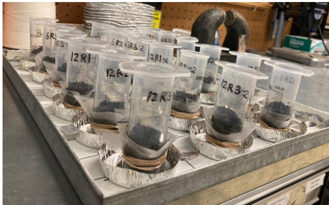
Figure 3. Polypropylene soil corers were used to take cores from the top inch of each column.
