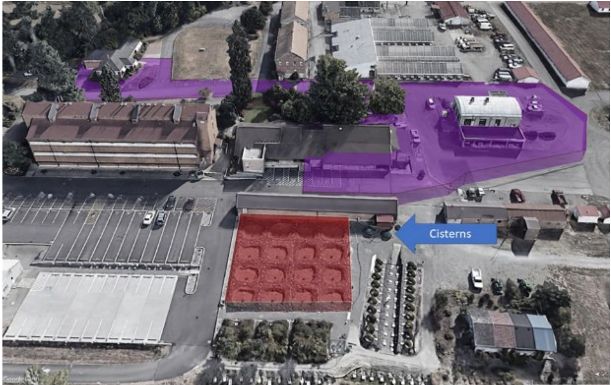
Figure 3: Image showing layout of facilities at WSU's Puyallup Research and Extension Center. Stormwater captured from a drainage area (purple) will be stored in a cistern, that in turn will be used to dose 16 bioretention cells (red area)
