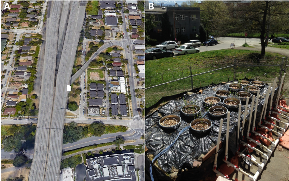
Figure 2. A) Location of study site under northbound I-5 in Seattle (small white rectangle). B) Bioretention cells surrounded by fill for thermal inertia, showing white standpipes and underdrains on right.
