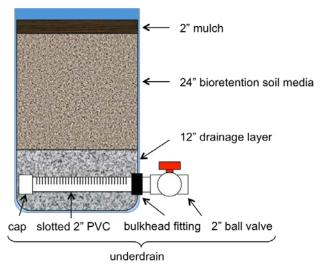
Figure 1: Schematic of the bioretention cell
