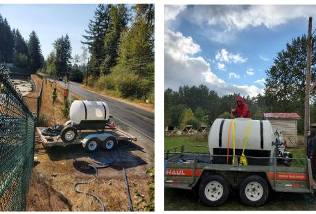
Figure 5: Hydroseeder used to spread plant seed.
