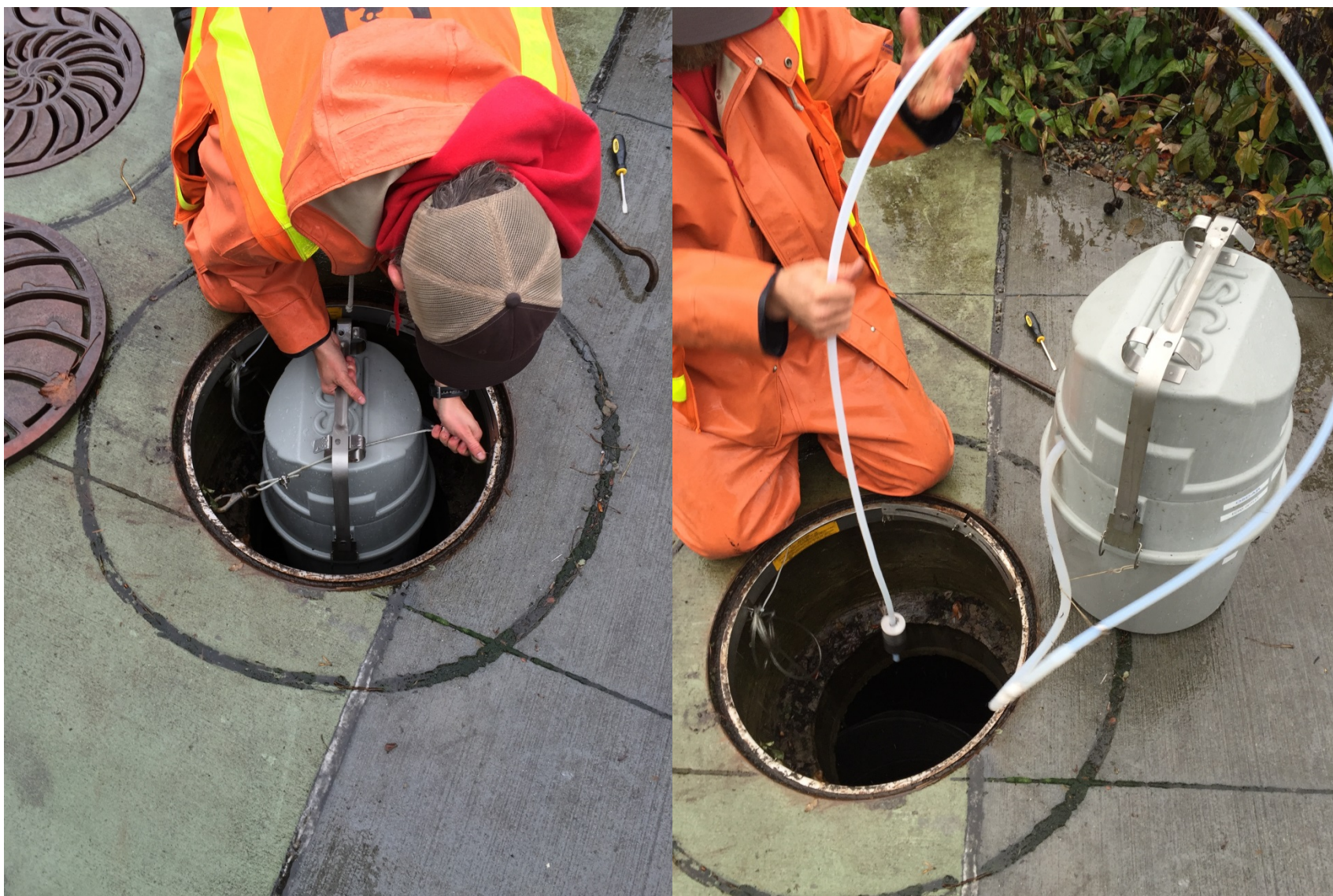
Figure C-6. DTS outlet sampling, ISCO autosampler retrieval, demonstrating weighted tubing (October 13, 2015).
