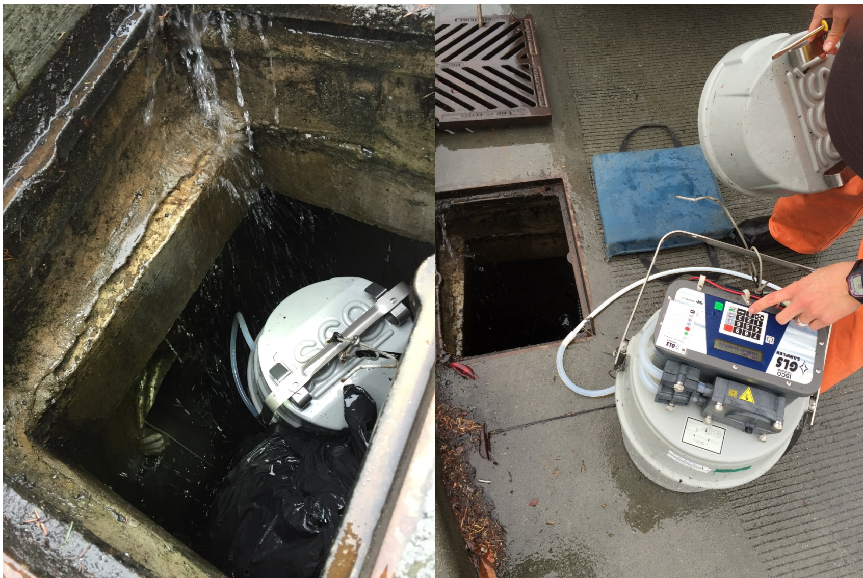
Figure C-5. DTS inlet sampling, ISCO autosampler retrieval (October 13, 2015).
