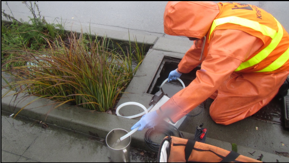
Figure C-3. BPB1 inlet sampling, peristaltic pump (December 8, 2015).
