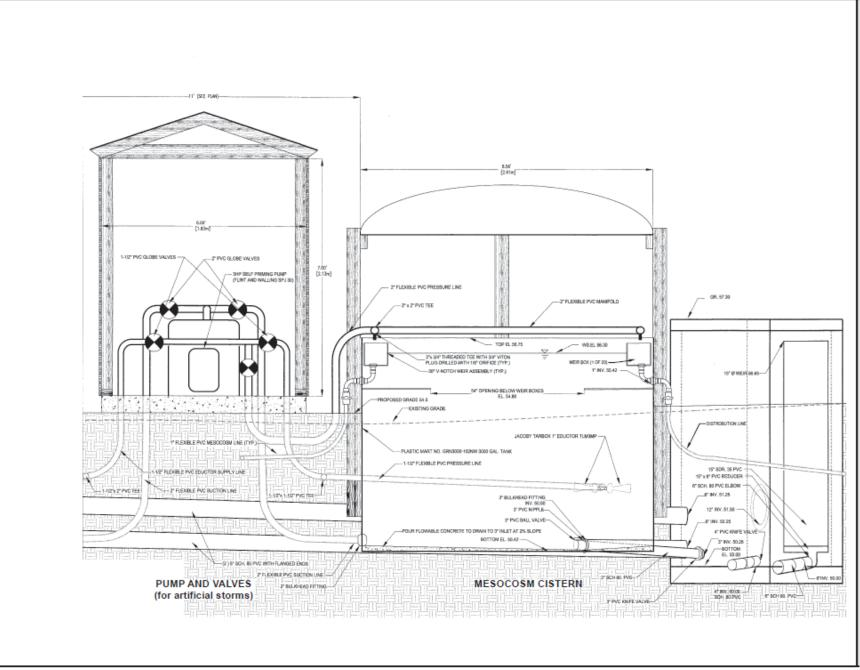
Figure 3. Schematic from the 2011 QAPP of existing pumping system, cistern, and piping.
