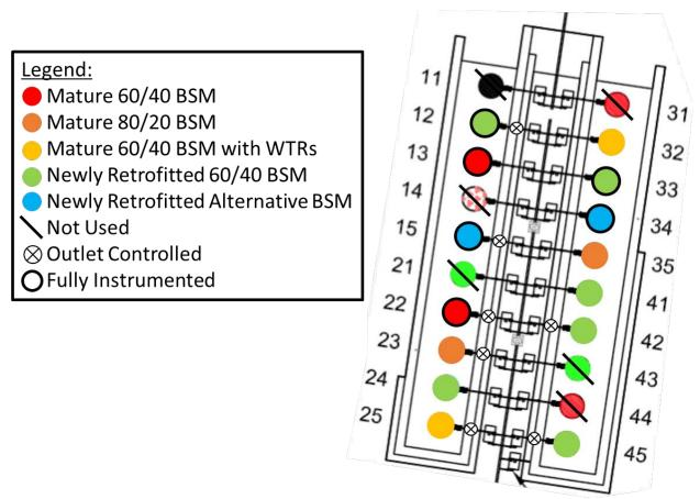
Figure 5.Mesocosms layout and modifications. Those mesocosms that are not used were found to have unacceptable leaking rates during a leak detection Site visit on March 17-18, 2020.
