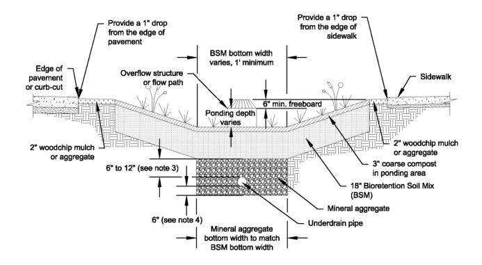
Figure 1: Typical design schematic for bioretention swale from 2019 SWMMWW).
