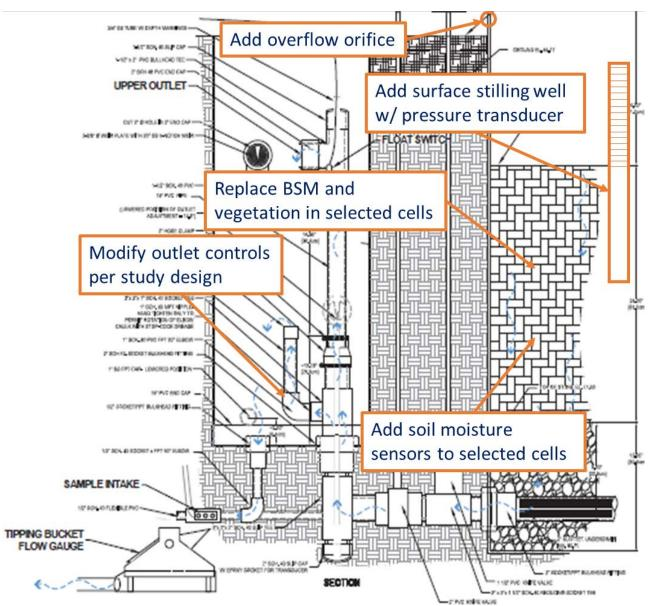
Figure 4. Schematic of mesocosms with proposed modifications.
