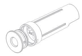
5. Turn the shuttle over and tap it gently. The circuit board should slide into your hand.
