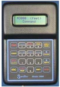
The Model 3000 Indicator is a datalogging version of the Model 2100, allowing the operator to input all measurement data usually kept on a clipboard while crossing a stream. The Model 3000 records depths, widths, velocities and angles along with time & date of measurements. It figures the "Q" and can upload all this information in spreadsheet-acceptable format to your PC for further study and
