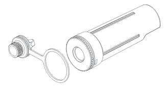
Turn the large cap counter-clockwise slightly, then pull it off.
