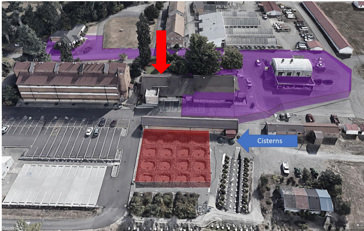
Figure 4: Image showing layout of facilities at WSU's Puyallup Research and Extension Center. Stormwater captured from a drainage area (purple) will be stored in a cistern, that in turn will be used to dose 16 bioretention cells (red area)
