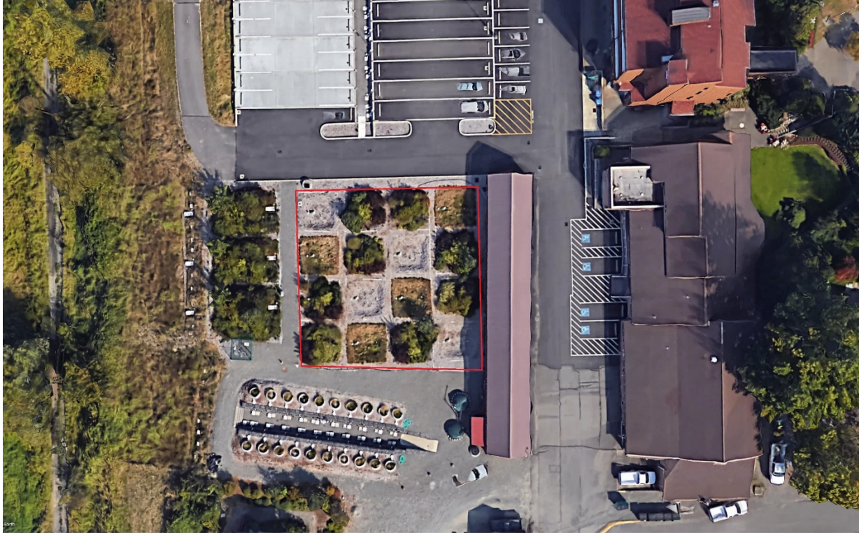
Figure 3: Layout of 16 bioretention test cells at WSU's Puyallup Research and Extension Center
