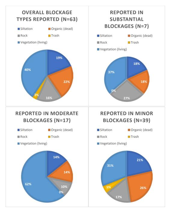
Figure 1: Types of inflow blockage reported during phase 2 Assessments. In phase 2 we divided out organic blockage types into living organic (vegetation) and dead organic (e.g. leaves and branches). Minor blockage is <5% blocked, moderate blockage if 5-50% blocked, and substantial blockage is >50% blocked.
