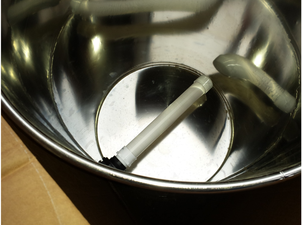
Figure 7-A. Stainless steel mesocosm barrel showing slotted screen underdrain pipe.
