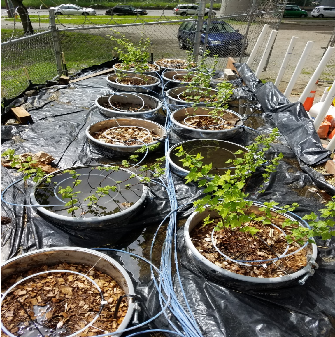
Figure 2-B. Flooded mesocosms with hydraulic conductivity standpipes shown in the upper right.
