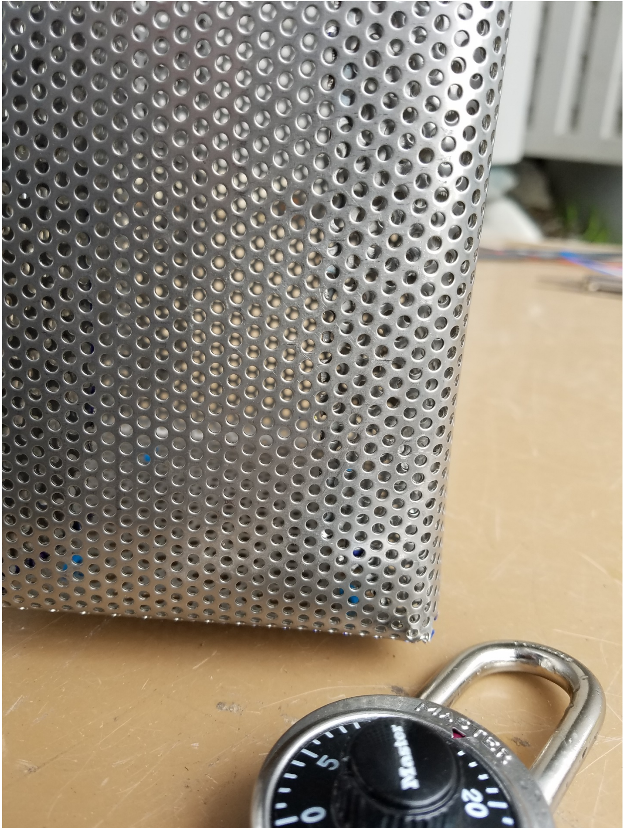
Figure 3-A. Screening used to pre-filter the dosing pump inlet to minimize clogging.
