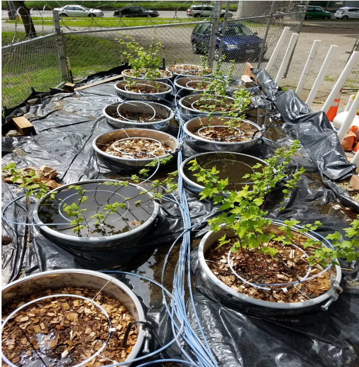
Figure 10-A. Mesocosms in May 2017. Flooded mesocosms were caused by inappropriate hydraulic conductivity testing methods initially used by project partners.
