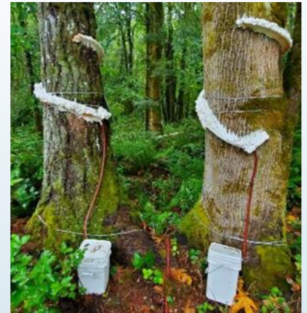
Mature trees were outfitted with sensors to measure tree transpiration and interception of rainfall
