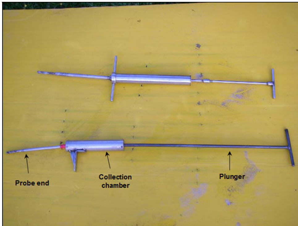
Photo 12. Syringe apparatus used to extract intergravel water samples. The narrow probe end is inserted into the gravel with the help of the foot pedal, to its full length. The plunger is pulled, drawing the water sample into the collection chamber.
