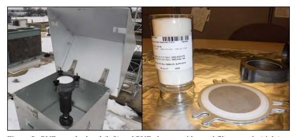
Figure 5. PUF sampler head (left) and PUF glass cartridge and filter sample (right).
