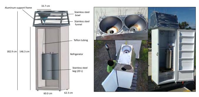
Figure 3. Schematic and Pictures of Bulk Deposition Sampler.
