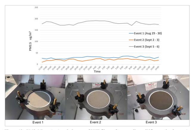
Figure 13. PM2.5 Data (top) and pictures of PUF filters after sampling wildfire smoke (bottom).
