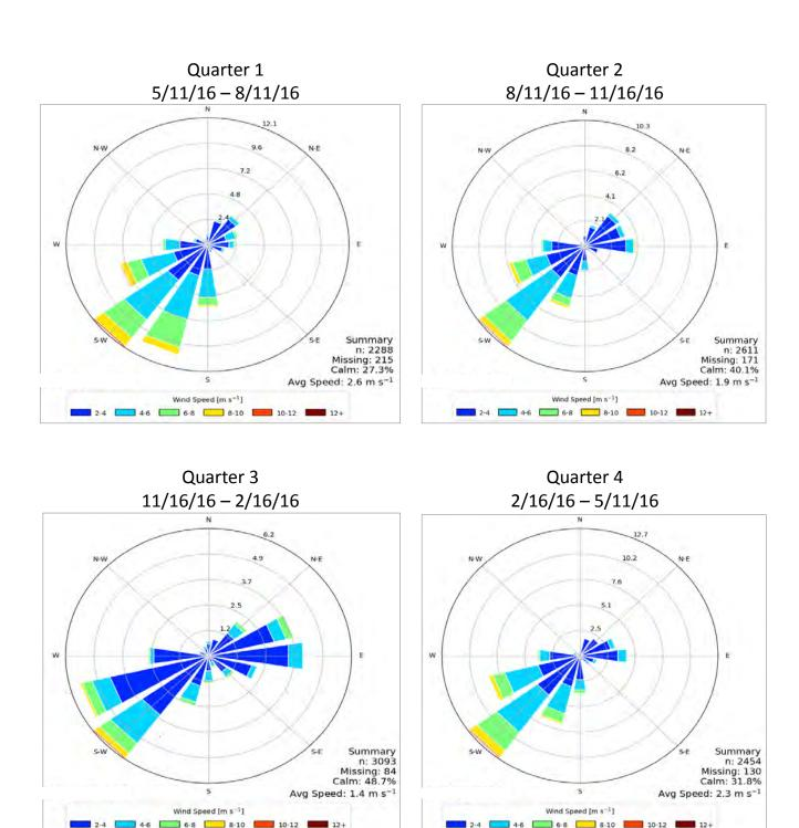
Figure C-3. Quarterly Wind Roses for the Felts Field Airport. *Calculated with Iowa State University online products using ASOS hourly data*.
