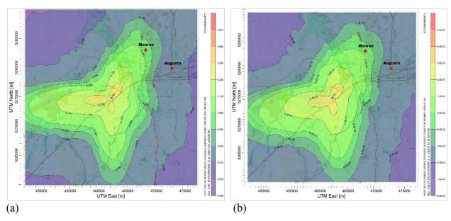
Figure 15. Modeled average annual PCB concentration distribution from the Spokane WTE stack. (a) For May 11, 2016 to May 11, 2017 field measurement case study. (b) Regulatory 5-year modeling study period of January 2011 to December 2015. Coordinates are in UTM (m) and concentration is in picograms per cubic meter ( $pg/m^3$ ).
