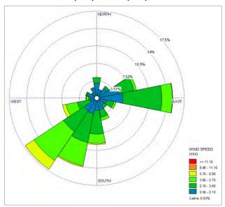
Figure C-1. Quarterly Wind Roses for the Augusta Ave. Monitoring Site. *Calculated with AERMET wind rose products using Onsite data*.
