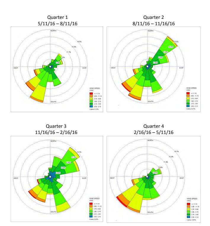
Figure C-2. Quarterly Wind Roses for the Spokane International Airport. *Calculated with AERMET wind rose products using ASOS 1-minute data*.
