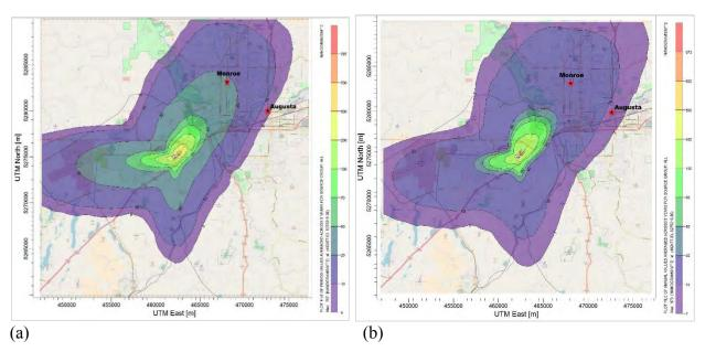
Figure 16. Modeled average annual total (bulk) deposition distribution from the Spokane WTE stack. (a) For May 11, 2016 to May 11, 2017 field measurement case study. (b) Regulatory 5-year modeling study period of January 2011 to December 2015.
