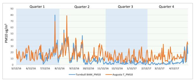
Figure 11. Daily average particulate matter <10 microns at the Turnbull and Augusta air quality monitoring stations.
