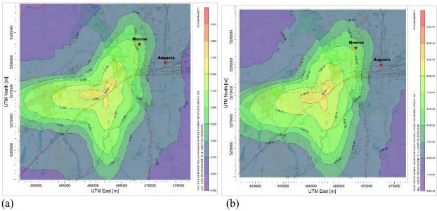
**Fig. 5**. Modeled average annual concentration distribution from the Spokane WTE stack. (a) For May 11, 2016 to May 11, 2017 field measurement case study. (b) Regulatory 5-year modeling study period of January 2011 to December 2015. Coordinates are in UTM (m) and concentration is in picograms per cubic meter (pg = picograms =  $10^{-12}$  grams).
