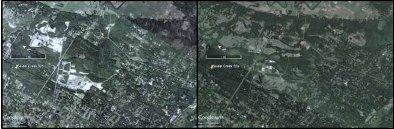
Figure F8. Aerial views of Seidel Creek watershed from 2002 (left) and 2014 (right). Imagery from Google Earth. Over one-half square kilometer (133 acres) of this 3.5 km 2 watershed converted to urban land cover during the decade 2001-2011.
