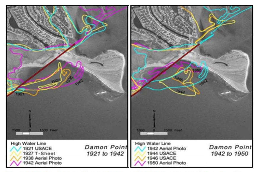
Figure 3-23. Evolution of Damon Point sand spit between completion of north jetty in 1916 and reconstruction in 1942, and post-reconstruction shoreline response by 1950
