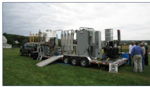
FarmBio3 Mobile Fast Pyrolysis Unit Source: USDA-ARS Fast Pyrolysis Team
