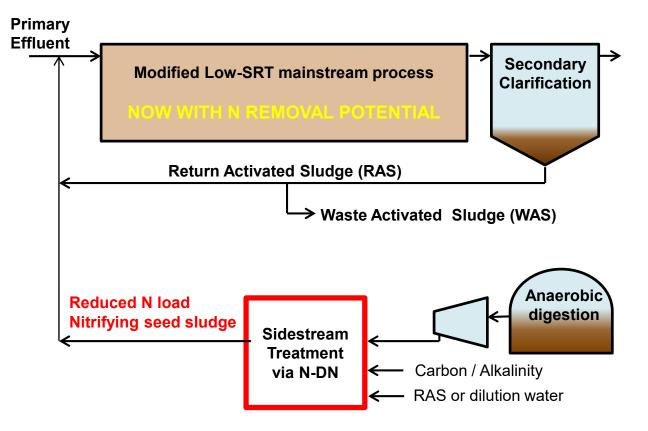
Parallel / Split treatment approach provides N removal and nitrification bioaugmentation potential
