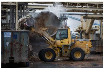
A heavy-equipment operator picks up garbage ejected from the pulping vat at NORPAC in Longview. The garbage was mixed in with the paper and cardboard that are being recycled. Twenty truckloads of... (Ellen M. Banner / The Seattle Times) **More** V
