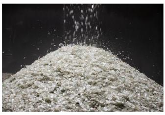
Crushed glass called cullet drops off a conveyor belt onto the apex of a 15-foot-high pile at Strategic Materials in Seattle. The Sodo facility sorts, cleans and tumbles fragmented glass from... (Ellen M. Banner / The Seattle Times) More V
