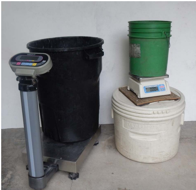
Photo taken July 24, 2019. Photo shows scales, buckets and cans used for 2019 residuals study.
