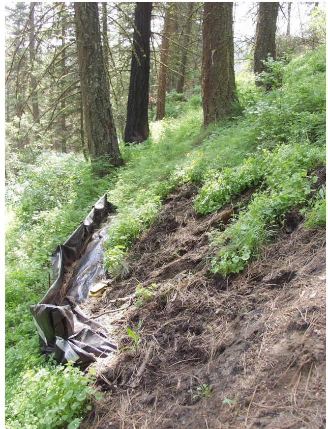
Figure 8. Red Fir project area, Cabin Gulch south, plot #6, a south-facing mid slope plot. Note the obvious bioturbation caused by elk walking above the sediment fence when the ground was wet, accumulation of sediment, short delivery distances, and damage to the sediment fence.
