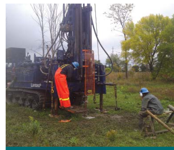
Figure 5.2.1: A drill rig being used for a geotechnical investigation. On a busy site, consider how the public will interact with drilling activity. (Source: Aquafor Beech)
