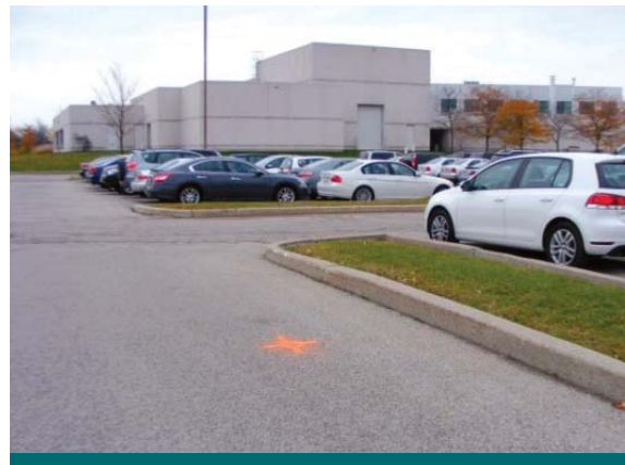
Figure 5.4.2: A neon mark indicates a borehole location. Consider how this borehole location will impact day-to-day operations on your site. (Source: Aquafor Beech)
