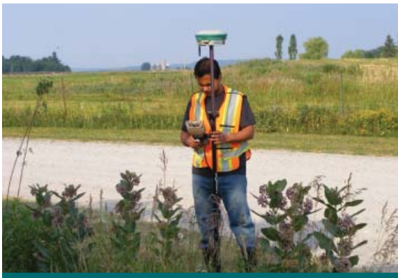
Figure 5.4.1: Topographic surveys ensure catchment areas are properly defined. Sites with flat catchment areas require high-precision equipment with GPS capability. (Source: Aquafor Beech)
