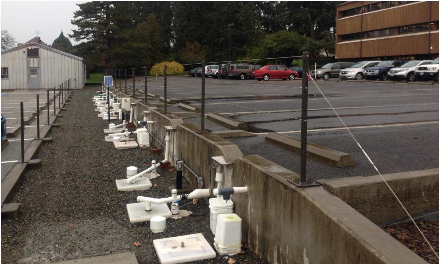
Figure 2. Permeable pavement tests at WSU Stormwater Center in Puyallip.
