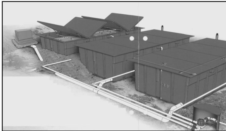
Figure 4: AdvanTex Systems (Courtesy: Orenco)
