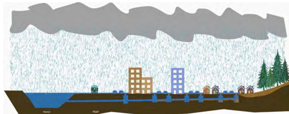
Current flood infrastructure leading to flooding from the river and due to system backflow. Note sediment coming down from hills, filling catchbasins, and high tide preventing conveyance from drainage pipes.
