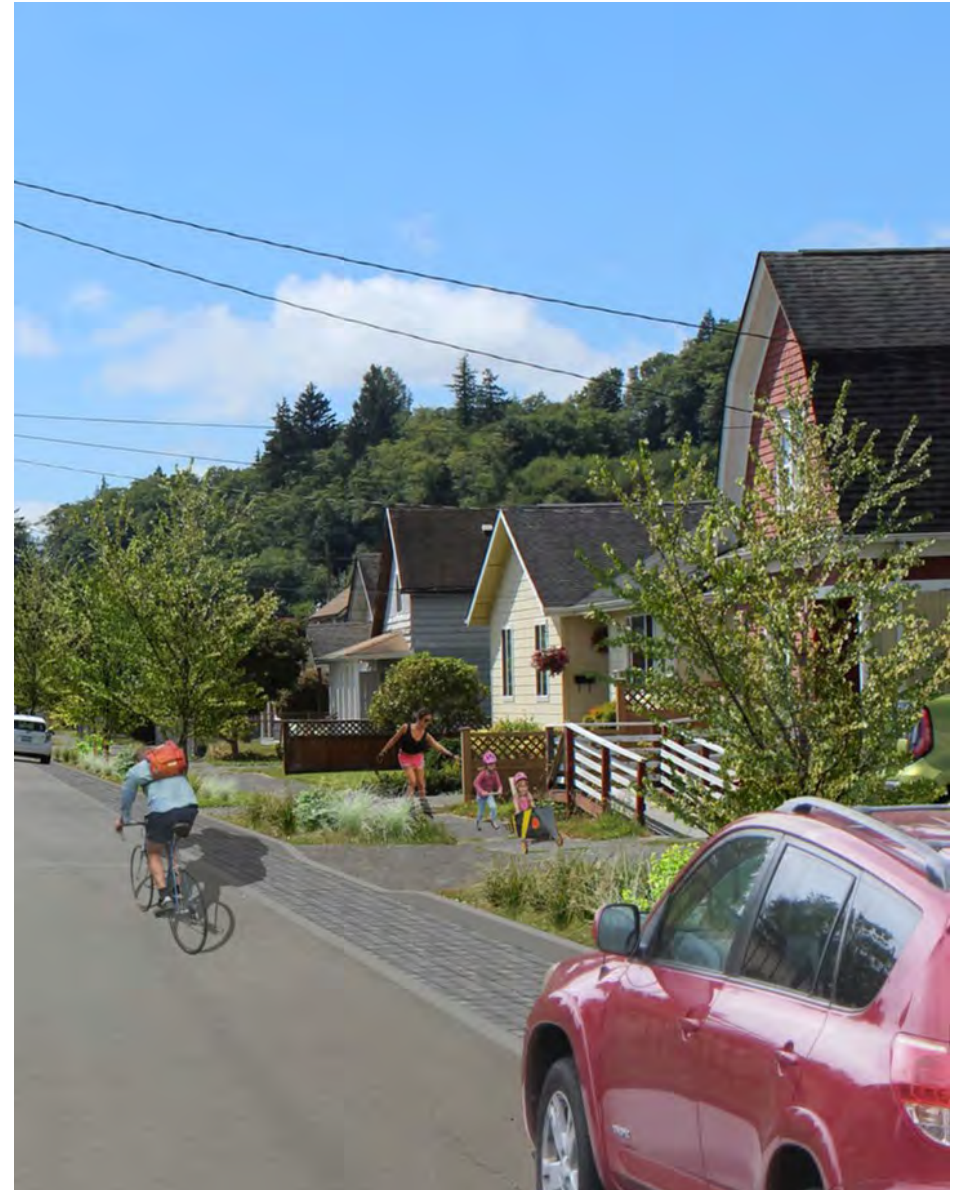
Illustration of 'green street' retrofits to Cherry Street including bioretention facilities and pervious pavement
